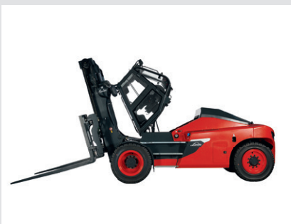
Engine access through tiltable cabin
