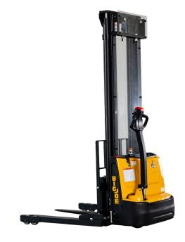
ergonomic operator handle. All operator controls are accessible without having to remove hand from the handle.
