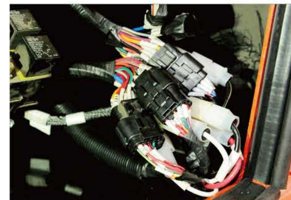
■ Dust proof and water proof sockets and plugs: protection degree IP65
