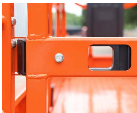
Self-locking platform door for operator safety.
