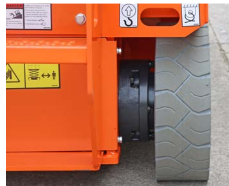
Front wheel hydraulic dynamic braking eliminates sliding while working on slopes.
